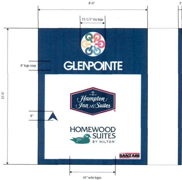
ELEVATION DETAIL SCALE: 1/2" = 1' logos will be routed and push-thru/ white acrylic small copy will be applied vinyl- colors TBD
